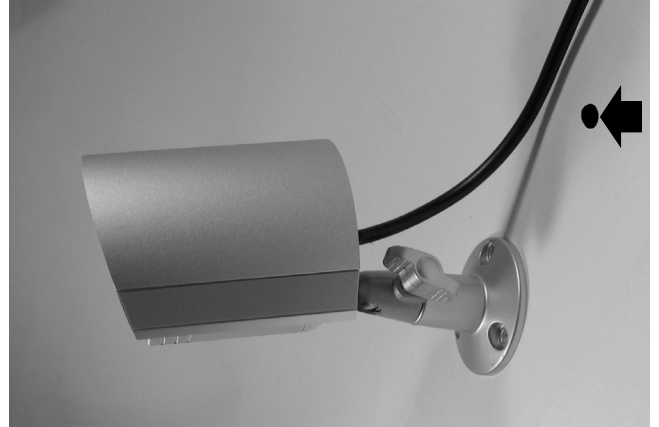
Fig. 3: Mount directly to a wall. Drill a hole in advance for the power and video cable to pass through later (arrow).
